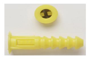
Plastic anchors are designed for use with lightweight fixtures. It can be used in concrete, block, brick, & wallboard. Holding values in wallboard tend to be inconsistent. Plastic anchors are injection molded from high quality polypropylene and designed to be used in conjunction with a sheet metal screw.
